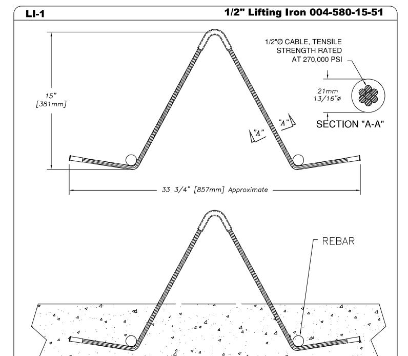
Lifting capacity rated up to 9800 lbs. per lifting iron.
