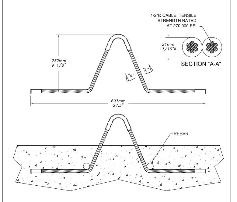
Lifting capacity rated at 14,000 lbs. per lifting iron.
